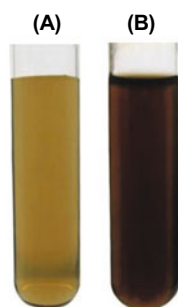
Fig. 1. Visible observation of AgNPs biosynthesis by S. viridochromogenes : (A) cell-free supernatant, (B) After exposure to (1 mM) \text{AgNO}_3 solution.
